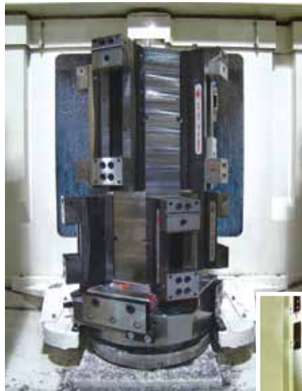
MTT-21 designed special fixtures for Schultes’ Kitamura Mycenter-HX400iF HMC to provide appropriate spacing between the manually operated vises and enable adequate clearances for the array of tools applied (inset).
