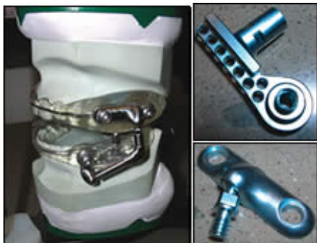
The titanium components of this assembled orthotic device are visible in this photo. The smaller photos show two of the individual machined parts from this assembly.
