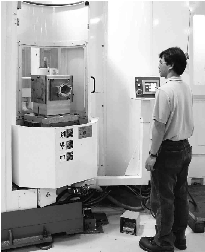
Chuong To loads and sets scheduling at the Kitamura HX400i load station.
