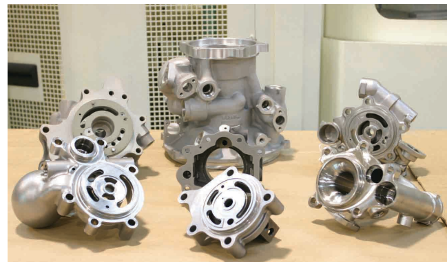
Complex hydraulic pump components produced on the Kitamura. Once such parts are produced, no more setup or first article inspection is required for subsequent orders.
