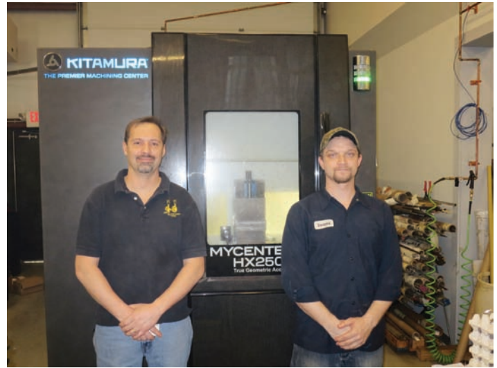
(l-r) Dan Labonville, President and Dwayne Dunton, Crucial Component Machining LLC, Concord, NH, with the Kitamura Mycenter-HX250G horizontal machining center that has a super compact, small footprint.
