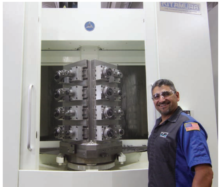
CP-Carrillo Supervisor Rigo Vargas and the tombstone design used with the Kitamura machines. This allows for more parts per load and provides access to more machining angles.
