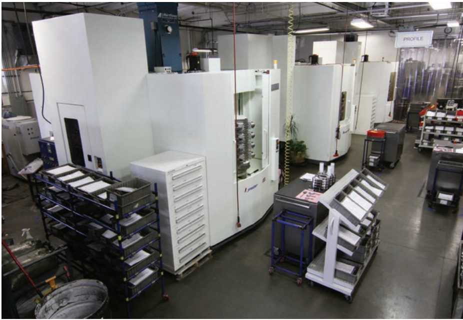
Optimized workflow in the Kitamura aisle of the Profile Machining Department at CP-Carrillo. CP-Carrillo has two Mycenter-HX400IFTGA (400 mm) and three Mycenter-HX500iTGA (500 mm) horizontals.
