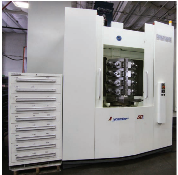
CP-Carrillo utilizes Kitamura machines for complex multi-angle large part machining using multi-part tombstone fixturing.
